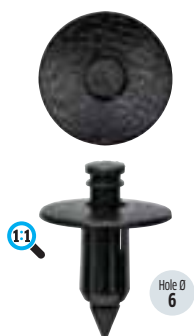
Black Windshield Push Rivets Ø x S: 18 x 11.5 mm Part No. Pack of FIX781 20 Nissan 8099905N07 Toyota 9046707043 / 9046707043C0 Volvo 987789
