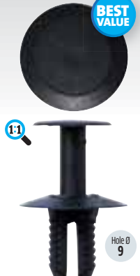
Black Push Rivets Ø x S: 20 x 14 mm Part No. Pack of FIX506 50 BMW 51471911992 Merc A2019900292 Mitsubishi M8201411 Volvo 30820141
